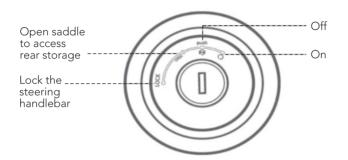
To lock the handle, turn the steering handlebar to the left then push the key inward and turn key anticlockwise to LOCK position
